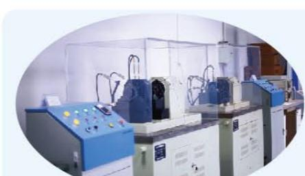
It is used for measuring the bearings defect by high frequency acceleration & vibration measurement,It can analysis the domain waveform,FFT frequency to analyze the reason part failure,through the detection of the instrument,It can check out for the bearings fault produced during the first production process,so as to guarantee the bearings long lifetime
